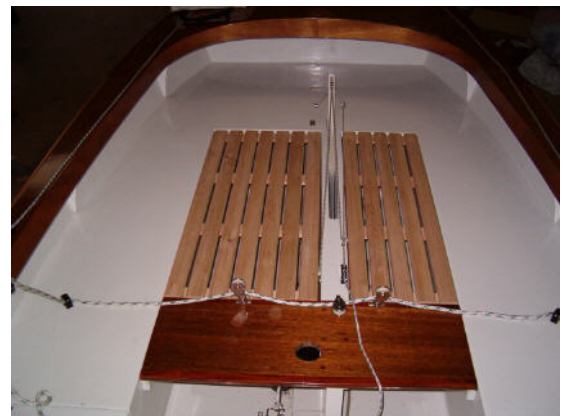
Optional, convertible floorboards, in the forepeak, are down during the day and up at night to make a large bed.
